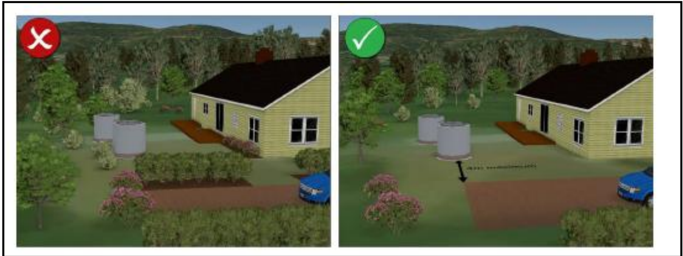
Figure 10: A good and a bad example of landscaping around a water tank and associated hardstand areas (WAPC, 2021)
