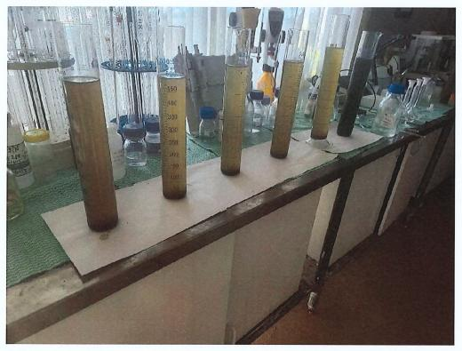
The first samples are shown in the photograph, with the untreated sample on the left with all samples settling out after 4 hours.
