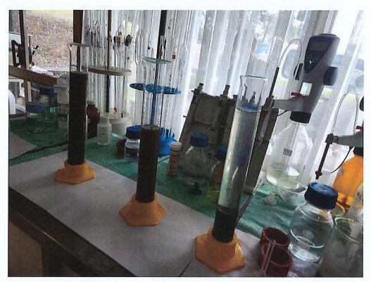
In the above photo of a later test, the sample on the right shows settling achieved with the addition of Ferric Chloride.
